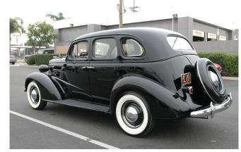
Chevrolet four-door sedan. It was totally black on the exterior and, inside, had some sort of beige material over horsehair-stuffed cushions. Its solid construction reminded me of an army tank: heavy steel frame and shiny steel bumpers, front and back, and "running boards," along the sides. The long-handled stick shift mounted between the two front seats was a challenge but, with practice, it handled the gears smoothly.
